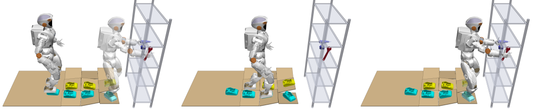
(a) Grasping a drill and a wrench in a shelf compartment on complex terrain with multiple support regions at different inclinations.
