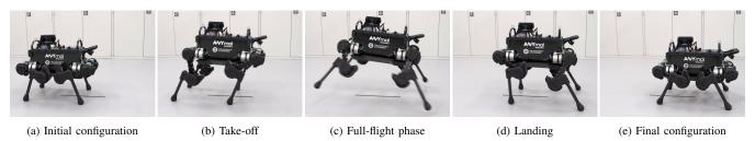
Fig. 4: Snapshots of ANYmal [27] performing a 0.5 m-long jump. The length of the black tape on the ground is 0.5 m.
